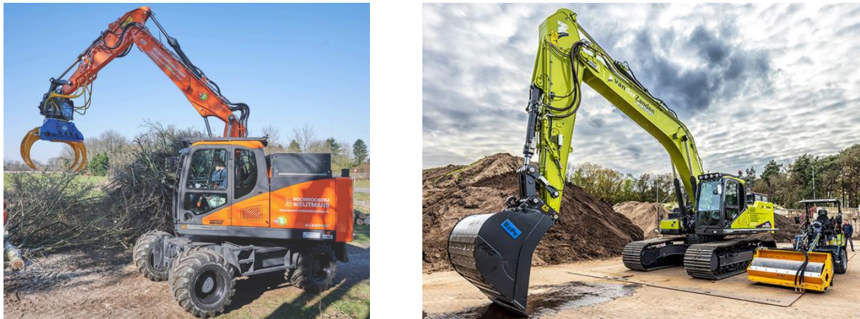
Figure 1: Left: 17-ton mobile excavator (type DX165W); right: 35-ton tracked excavator (type DX355LC)
