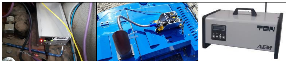
Figure 4: Measurement equipment; left: SEMS CAN/sensor data logger, middle: portable NO x emission measurement system, right: portable particulate matter measurement system.
