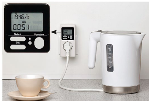
Figure 7: Experiment on measuring power and energy consumption of an electrical device from the physics textbook [8]
