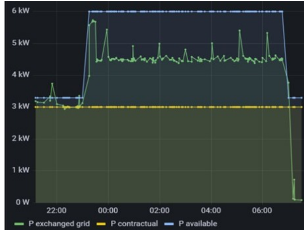
Figure 1: Flexible connection agreement for EV owners: charging operation at nighttime that exploits the extra available power from 3 up to 6 kW. (Image courtesy from [14]).
