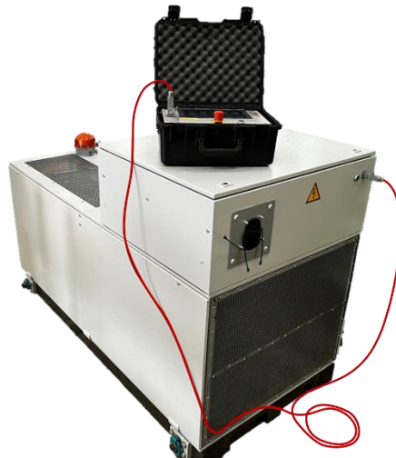
Figure 2: ProSafeE 2 testing device demonstrator with fiber-connected external control unit
