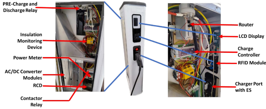
Figure 10: Hardware setup of the 45kW modular and scalable charger container.;
