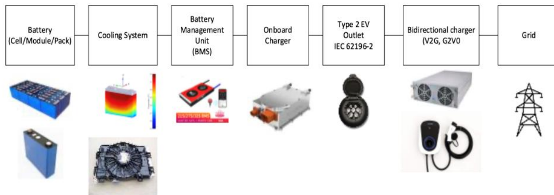
Fig.3 V2G Charging system
