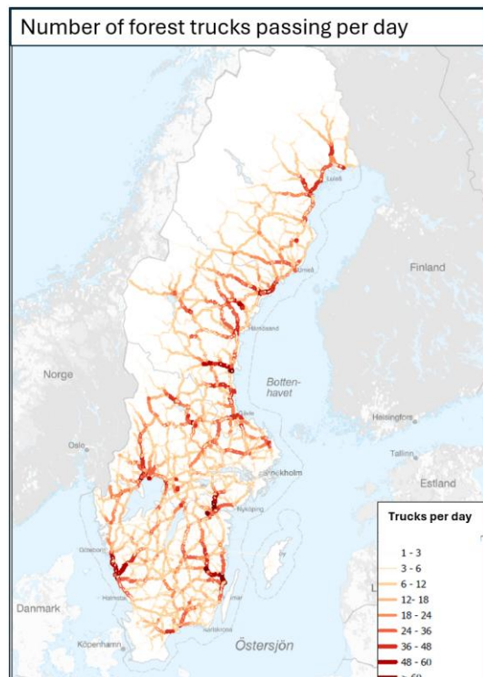
Figure 5. Transport intensity translated to number of forest trucks passing per day for different road sections.
