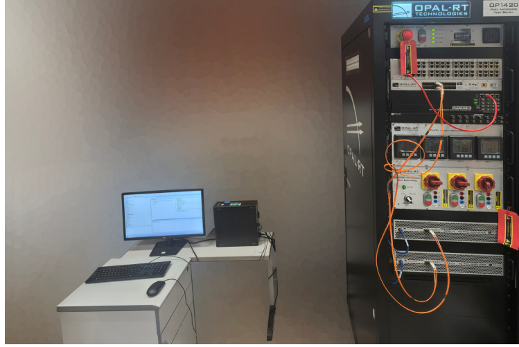
Figure 4: OPAL-RT power-hardware-in-the-loop (PHIL) simulation system.
