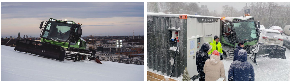
Figure 8. Electric snow groomer used during the fossil free ski resort pilot in Stockholm. (left) in the slope, (right) by the charger
