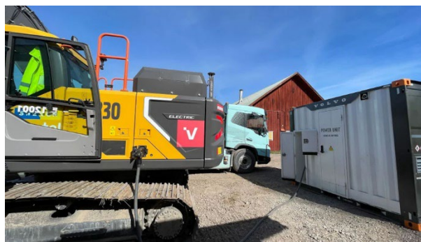
Figure 6. Electric truck and excavator charging from BESS to enable zero emission operation in a temporary location with limited grid supply.
