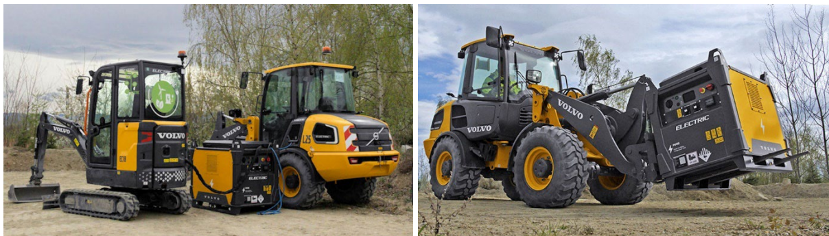
Fig 1. A 40 kWh ‘Power Unit’ for charging compact construction equipment as well as for powering other site tools.
