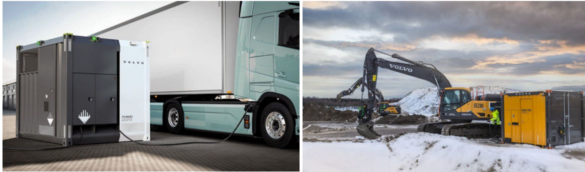
Fig 2. (left) A recently launched 500 kWh ‘Power Unit’ which enables fast DC charging on low power grid connections. (right) Fast charging of an electric excavator at a construction site in Norway.
