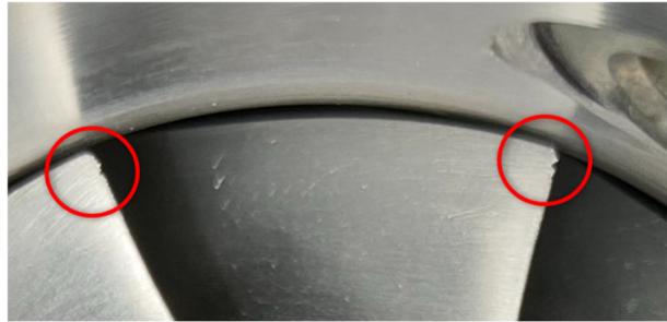
Figure 7: Erosion on compressor wheel due to droplet impingement
