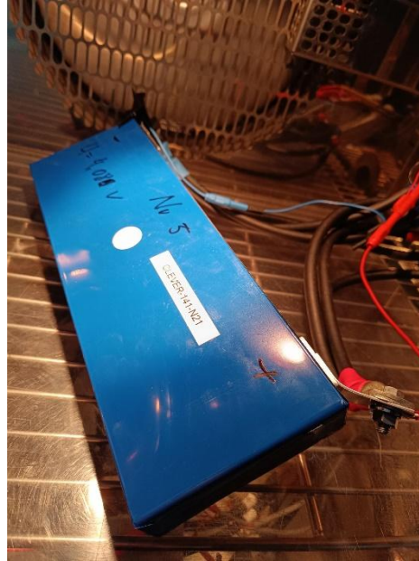
Figure 1: Sample pouch (left) and prismatic (right) cells setup for aging tests.
