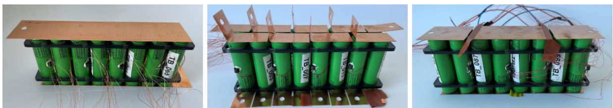
Figure 3: Assembled modules in 2x8 topology (1s16p, 16s1p, 4s4p)
