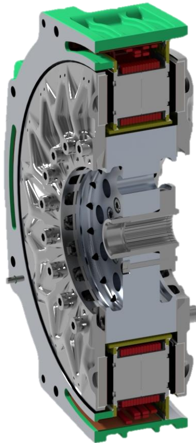
Figure 1: CAD rendering of the axial machine stator and rotor cross section.
