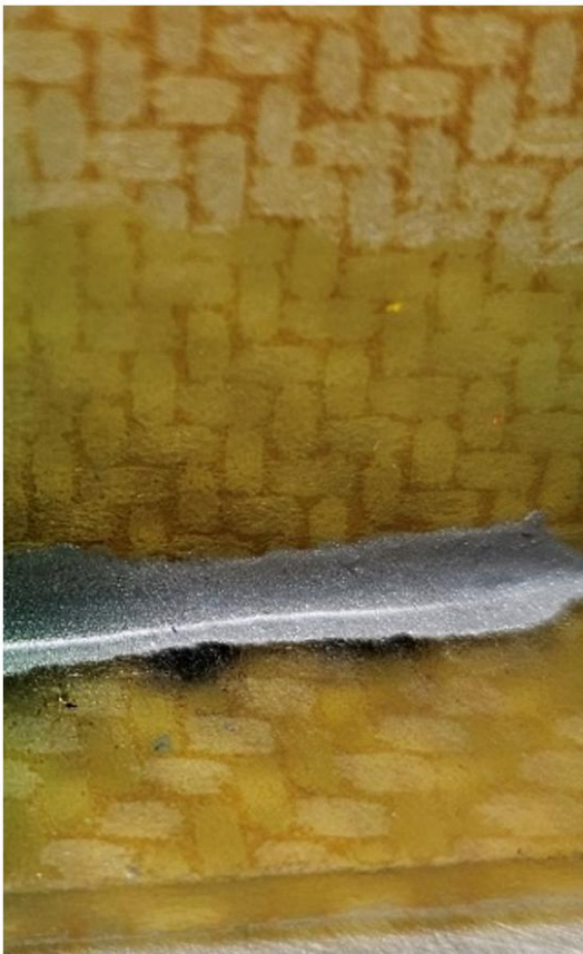
Figure 14: Adhesive joint on the upper side (left) and the underside (right) after curing with 0.10 mm glue gap. The joint has a nice radius on the upperside, has penetrated the glue gap fully and formed a small radius on the underside.
