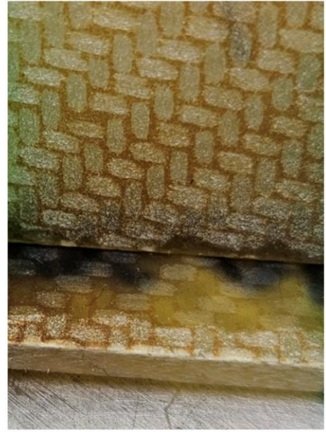
Figure 13: Adhesive joint on the upper side (left) and the underside (right) after curing with 0.05 mm glue gap. The joint has a nice radius on the upper side but has not fully penetrated to the underside.
