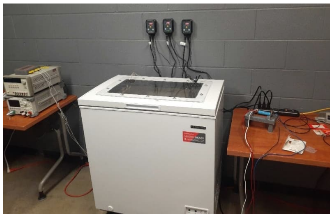
Figure 2: Cell Tester Temperature Control Chamber
