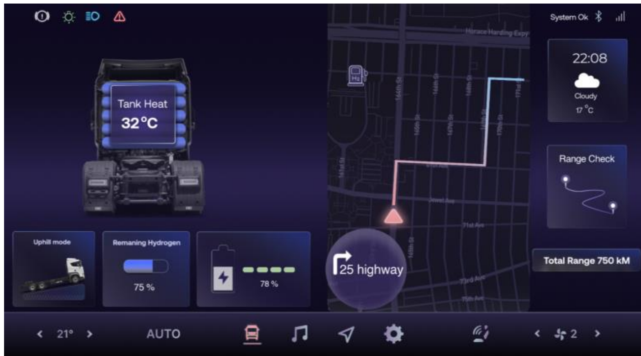
Figure 2. f -HMI main interface showing hydrogen fuel levels, auxiliary battery status, nearest H2 refueling station, and route with range estimation.
