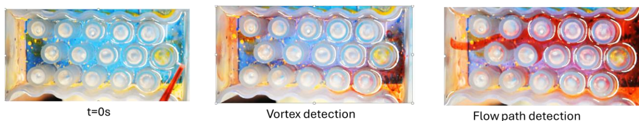
Figure 12: Visualization of the direction flow using colored tracer
