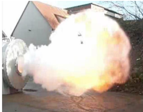
Figure 2: A vented dust explosion in an industrial-scale vessel, used under Creative Commons CC-BY license [11].
